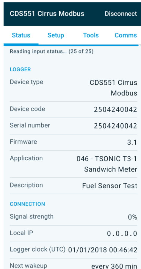
Figure 4. Connected: the setup is read automatically, with progress under the tabs
