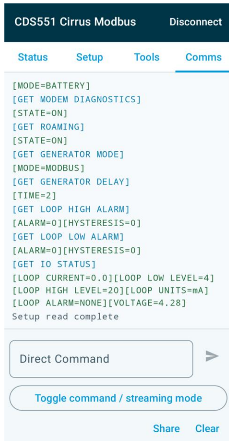
Figure 22. Comms after a setup read: commands and replies in brackets
